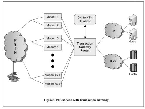
As shown in above figure, if the transaction terminal dials a unique number identifying the credit provider, a Total Control system using the Transaction Gateway can map this telephone number (using DNIS Feature Group B or D) to a particular X.25 address or TCP host and port number.
