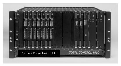
**Modular Architecture:** The platform includes intelligent Network Application Cards (NACs) in front of the platform where they can be easily swapped and Network Interface Cards (NICs) in back where cabling is secure and out of the way.
